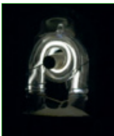
Picture 3: As the resistance drops, the tube fills up with xenon, which is now in a plasma state.
