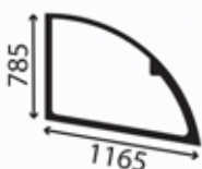
Window, cabin side RH; front; flat; green tinted
