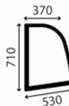
Window, cabin side LH; rear; flat; green tinted
