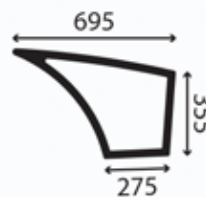
Window, cabin RH door lower Flat; green tinted
