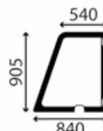
Window, cabin LH door upper Opening; flat; green tinted Used on machine type: A REF 164TA3989
