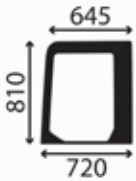
Window, cabin LH door upper Curved; green tinted
