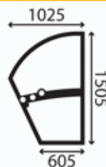
Window, cabin LH door LH; flat; green tinted Used on machine type: B, C, D, E, F, J, M REF 164TA5227
