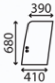
Window, cabin LH door upper LH; front; upper; sliding; flat; green tinted
