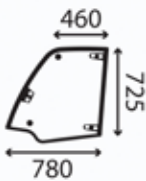
Window, cabin LH door upper Opening; flat; clear
