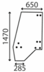
Window, cabin LH door Curved; clear; up to S/N M315336
