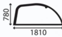
Window, cabin side RH; flat; green tinted Used on machine type: A, B, C, D, E, F, G, H, I, J, K, L, M, N, O, P, Q REF 166TA2355
