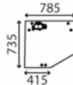
Window, cabin rear Flat; green tinted; big wiper motor axle at 180,00 mm from LH side; includes print for wiper motor
