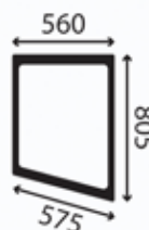
Window, cabin side RH; rear; flat; green tinted
