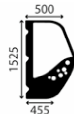
Window, cabin side LH; rear; flat; green tinted Used on machine type: A, B, C, D, E, F, G, H, I, J, K, L, M, N, O, P, Q REF 166TA2371
