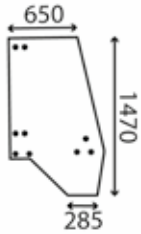
Window, cabin RH door Curved; clear; up to S/N M315336
