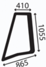
Window, cabin side RH; corner; curved; green tinted
