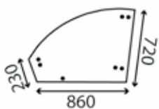
Window, cabin LH door upper Used on machine type: F, J, M REF 164TA5228
