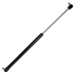
Gas spring, hood/cover 700 N; length: 685,00 mm
