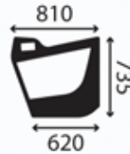
Window, cabin LH door lower Flat; clear
