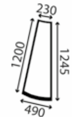
Window, cabin side LH; corner; curved; green tinted
