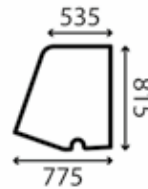
Window, cabin LH door upper Flat; green tinted Used on machine type: A REF 166TA2129
