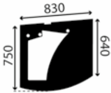
Window, cabin LH door lower Flat; green tinted
