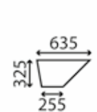
Window, cabin door lower
