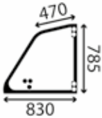
Window, cabin LH door upper Opening; flat; green tinted; thickness: 6,00 mm
