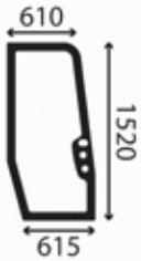
Window, cabin RH door RH; flat; green tinted
