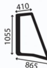
Window, cabin side LH; corner; curved; green tinted
