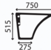
Window, cabin LH door lower Flat; green tinted
