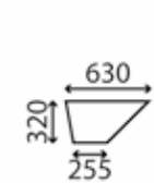
Window, cabin door lower Flat; clear; up to S/N M363331
