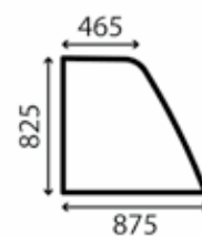
Window, cabin RH door upper RH; upper; flat; green tinted
