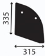
Window, cabin LH door lower LH; lower; flat; green tinted
