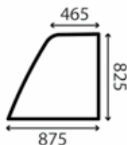
Window, cabin LH door upper LH; upper; flat; clear
