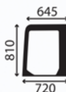
Window, cabin LH door upper Curved; green tinted
