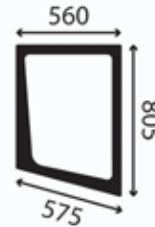
Window, cabin side RH; rear; flat; green tinted
